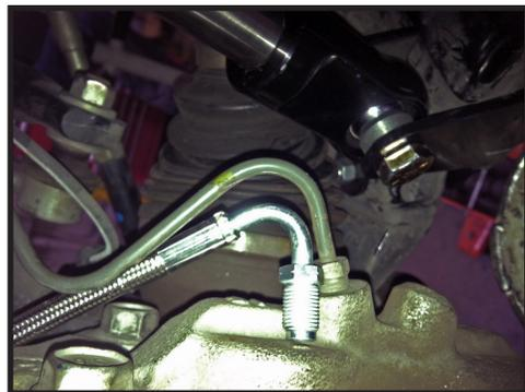
**19.** Remove the factory brake line routing bracket from frame and relocate it as pictured using a 1/4" drill bit and supplied 5/16" self-tapping screw. [Torque to 25 ft-lbs] (FIGURE 13)
