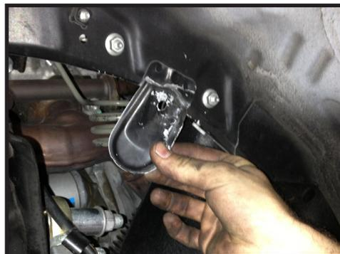
6. Some fender liners have a sheet metal tab that has to be removed and two screws protruding that need to be sanded flat to get the hoop to locate properly on the frame. (FIGURE 2)
