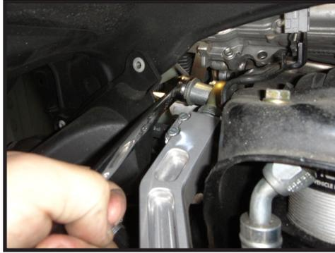
**8.** Install the taper pin adapter up into the uniball, install the upper dome on top and install the 12pt 1/2" bolt in the top. Make sure the radius of the taper adapter and upper dome meet the diameter of the inner ball of the uniball. Hand tighten the upper bolt for now. It will be torqued with thread locker later.
