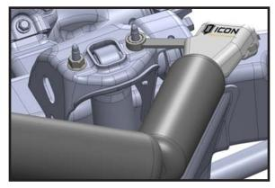
**3.** Before lifting vehicle to droop suspension, loosen and remove front (2) upper shock nuts. This will allow suspension to extend further when lifted. To access shock bolts fender well may need to be removed.
