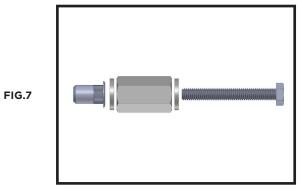
**9**. Insert the rivet nut in each hole and use the supplied rivet nut setter to crimp the rivet nut onto the sheet metal. Use a 1/2" to keep the coupling nut from spinning, tighten the 10-32 x 1.5" bolt using a 5/16" until the rivet nut sets. Remove the rivet nut setter. Repeat for all rivet holes. [FIGURE 8]
