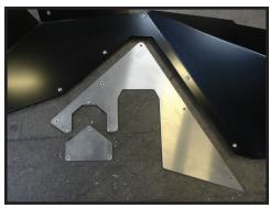
2. With factory fender liner removed, use the (2) factory screws and a 10mm to mount/hang the fender liner to the top of the fender. Tighten slightly. (Refer to Figure 2) Make sure the front vertical portion of the fender liner is on the outside of the fender and flush against it. [FIGURE 2 & 3]
