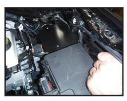
9. Remove the backing from the adhesive rubber strips and place them as shown. [FIGURE 9]
