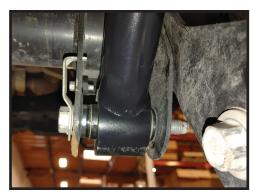
**19.** Re-install the OE lock nuts onto both the front and rear lower link pivot bolts. Use a 24mm socket and torque wrench to torque them to factory-recommended specifications.
