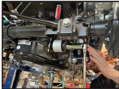
**16.** The rear lower link bolt nut has a long keeper tab, measure 1-1/4" from the end of the keeper tab and mark it. Use a cut-off wheel to cut at the mark. The result should be that the keeper tab (on the axle housing pivot bolt only) is 1-1/4" shorter, as shown on the left in. [FIGURE 16]
