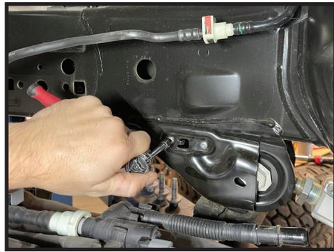
**14.** Use a 24mm deep socket and ratchet or driver to remove the nut from the lower link pivot bolt, frame end [FIGURE 14]. Remove the bolt while taking care to secure the link with a bungee cord, ratchet strap or the hand of a friend, as it may fall out of the link pocket once the bolt is moved.
