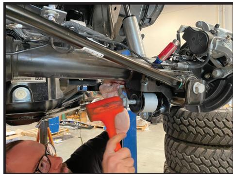
**19.** Re-install the OE lock nuts onto both the front and rear lower link pivot bolts. Use a 24mm socket and torque wrench to torque them to factory-recommended specifications.
