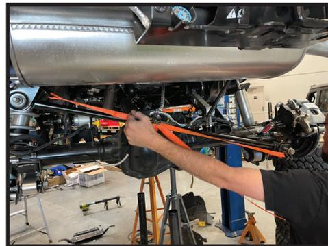
5. Install the passenger side lower link first, which will require lowering the fuel tank to access the frame-side pivot bolts. Begin by disconnecting the wiring harness from the rear of the fuel tank. The connector is located above the fuel filler hose.
