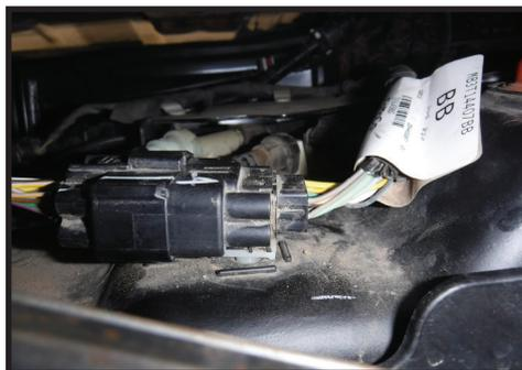
**11.** Near the top-front of the tank, use a body clip removal tool to pull the wiring harness retainer from the retaining hole in the tank (4-Door Bronco only) [FIGURE 10]. Dislodge the fuel line from the groove in the top of the tank. [FIGURE 11]
