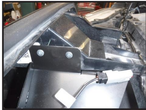
**8.** Connect the wire harness (PN: 255602) to the black plug on the IIC.
