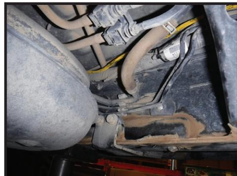
**26.** Plug into the driver rear CDE-Shock solenoid and zip-tie the remaining wire. Be sure to leave some slack in the wire to ensure there is freedom of movement and the ability to unplug the wire from the shock. [FIGURE 18]
