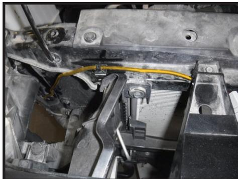
**16.** Route down into the passenger side fender well and connect to the passenger side CDE-Shock solenoid. Zip-tie any excess wire in the engine compartment in a safe/protected area [FIGURE 6]. Be sure to leave some slack in the wire to ensure there is freedom of movement and the ability to unplug the wire from the shock.
