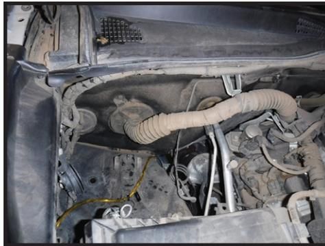
**18.** Route the wire along the top of the frame rail following the factory harness. [FIGURE 8 & 9]
