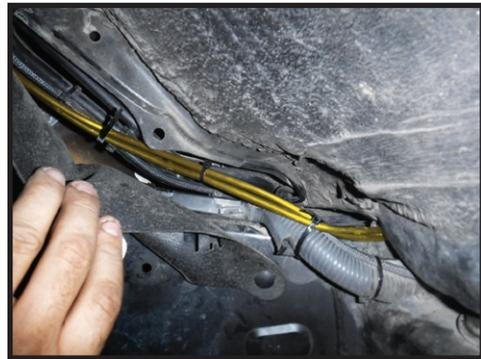
**24.** Pull the wire through into the back of the wheel well. Feed the wire back along the top of the driver side frame rail. Continue zip-tying as you go. [FIGURE 15]
