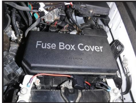
**30.** Remove the INJ Fuse and place it in the lowest slot of the supplied fuse tap (PN: 255607). Insert the supplied 2 AMP fuse (PN: 605754) in the upper slot. [FIGURE 20 & 20B]
