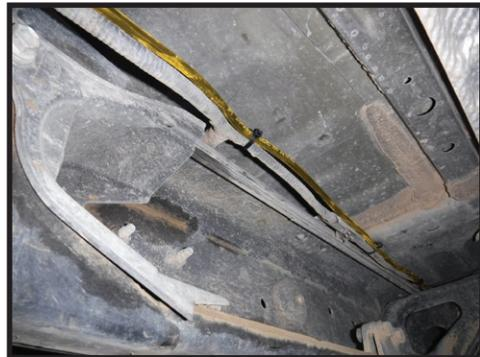
**19.** Connect to the CDEV shock and zip-tie excess wire up in a protected area. Be sure to leave some slack in the wire to ensure there is freedom of movement and the ability to unplug the wire from the shock. [FIGURE 10]
