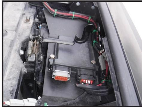
**10.** Use the supplied wire loom (PN: 605760) to hold the 2 black "Ground" wires and the Red "PWR/BATT" wire together. Slide the loom up close to the connector of the IIC. Route the loom between the fender and the fuse box. Trim as needed.
