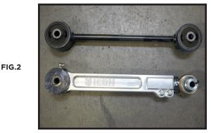
5. Install the link. The rod end mounts to the axle and the bushing mounts to the frame. Slide the bolt through the frame end first but do not tighten, next insert the bolt through the axle end.
