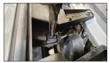
Use a flat screwdriver or body panel removal tool to release the clips that attach the headlights to the grille.
