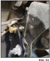
The two long spacers go inside the body mount perch, with the lock nut on the opposite end of the bolt. Use a flat washer under the head of the bolt and the lock nut. Extra washers are provided to use as spacers if needed to accommodate manufacturing variances from vehicle to vehicle.
