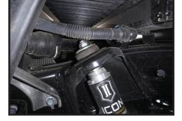
6. Install the lower eyelet of the Icon shock onto the axle stud. A deadblow hammer can be used to get the lower eyelet on the stud completely. Use the factory bolt and torque to factory specs. [FIGURE 4]
