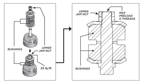
HEAVY DUTY STEM BUSHING DIAGRAM & ASSEMBLY
