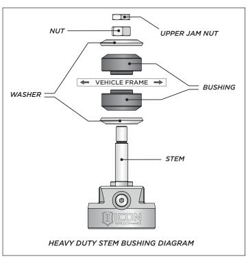
10. Tighten both the upper and lower stem nuts so that there are 4-5 threads showing through the nut. Install the jam nut on both ends and torque to 35ft\*lb. (See diagram)
