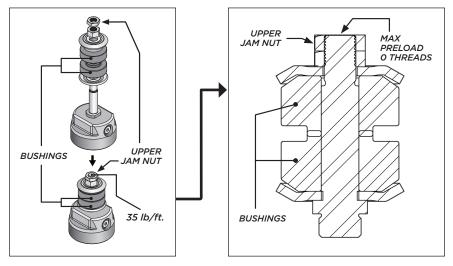
HEAVY DUTY STEM BUSHING DIAGRAM & ASSEMBLY
