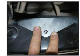
10. Using the hole in the bracket as a guide, center punch and drill to 21/64".
