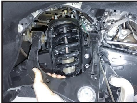
**21.** Install the new bushings into the ICON tubular UCA as indicated by the drawing below. Grease the ID and OD bushing and the face before install. [FIGURE 21]
