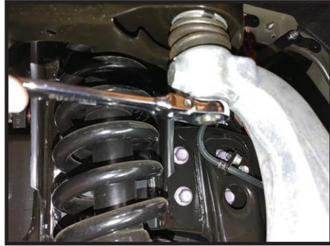
**16.** Use a hammer or balljoint separator to loosen the balljoint taper from the spindle. [FIGURE 15]
