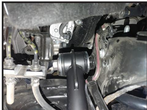
**23.** Install the Delta Joint Pro into the spindle, apply included blue thread locker to threads on flange nut and thread on to Delta Joint Pro with washer (PN 605890) between the flange nut and spindle [Torque the nut to 70 ft-lbs]. [FIGURE 24]
