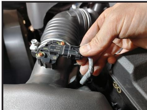
**5.** Remove the airbox. Loosen the hose clamp with a #2 phillips screwdriver or 10mm on the air intake hose located closest to the engine. [FIGURE 2]
