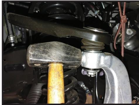
**17.** Loosen and remove the UCA pivot bolt from the frame using a 22mm. [FIGURE 16]
