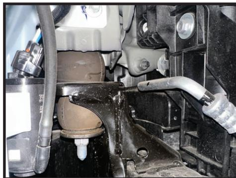
**19.** Using a jack carefully apply pressure to the driver front core support bolt this will lift the intercooler up enough to remove the UCA pivot bolt. [FIGURE 18 & 19]
