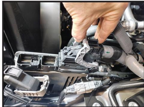
**10.** Remove the harness clamp from the large wire loom using a small flat blade screwdriver. [FIGURE 7]
