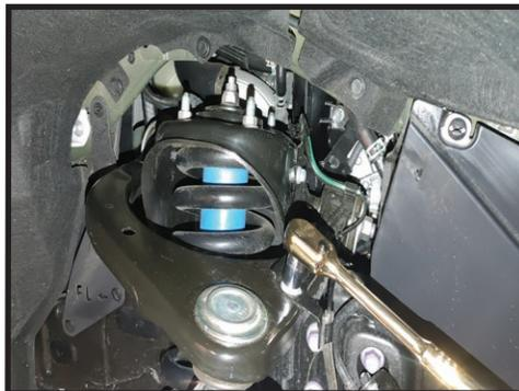
**15.** Remove the cotter pin from the UCA balljoint using a small screwdriver or pick to pry over the safety clip and pull out the pin using a needle nose pliers. Loosen the 19mm nut on the balljoint. [FIGURE 13 & 14]
