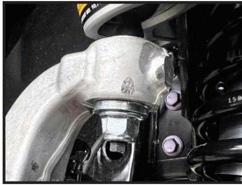
**24.** Install the ABS bracket onto the Billet UCA using the factory bolt. [FIGURE 25]
