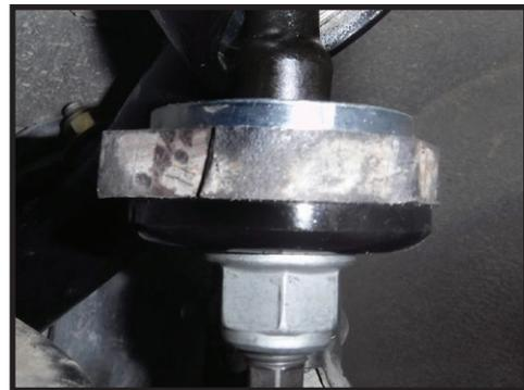
**8.** Install the Delta Joint on the Delta Joint Adapter. Make sure the taper of the Delta Joint fits properly in the Delta Joint Adapter. Install the bottom adapter plate and supplied nut. [Torque to 75 ft-lbs] [FIGURE 5 & 6]
