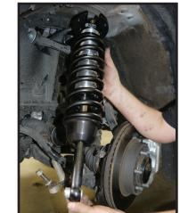
**9.** Connect the shock to the lower control arm: The lower shock mount has (1) long and (1) short spacer [Torque to factory spec]. Make sure the long spacer is toward the front of the vehicle as this will position the shock further toward the rear of the control arm to ensure adequate sway bar clearance. Install the factory lower shock bolt.
