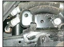
17. (KDSS ONLY) For vehicles equipped with Kinetic Dynamic Suspension System, each remote reservoir bracket will be mounted using two (605144) self-tapping bolts.
