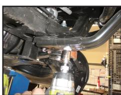
**5.** (NON KDSS VEHICLES ONLY) Disconnect the sway bar from the frame on both sides. Remove bolts using a 14mm socket/wrench and remove the bracket from the sway bar. Move the sway bar forward to make room for removal and installation of the shock.
