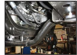
23. Slightly bend the hanger tabs down on the factory skid plate, they will no longer be used. [FIGURE 11]
