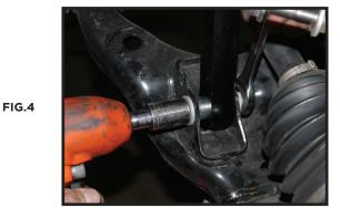
**12.** If replacing the upper control arms, refer to appropriate UCA instructions now. Mount the upper control arm to the knuckle and tighten the taper nut. [Torque to factory spec]
