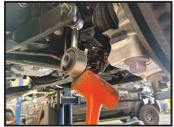
3. Loosen and remove the nut of the upper portion of the link using a 19mm. Remove the link from the swaybar and set aside with the nut.
