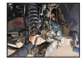
22. Grind/cut the lower shock pocket on the control arm to add clearance for the new ICON coilover assembly. Removing the control arm can help make this easier. If removed, be sure the bolts go back into the same place and orientation. After cutting is complete, paint over the raw metal to prevent rust. [FIGURE 21 & 22]
