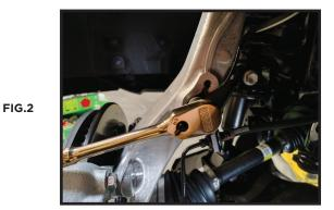
5. Remove the brake caliper from the spindle using a 19mm. Once removed, use a strap or rope to support the caliper so it does not hang by the brake line. Remove the brake rotor and set aside. [FIGURE 3 & 4]
