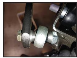
**38.** Install the lower end of the sway bar link onto the lower control arm stud. First the sleeve, then the link and second sleeve. Reuse the factory bolt and torque to factory spec. [FIGURE 31 & 32]
