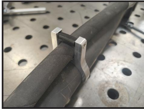
5. The reservoir hose should still move freely. Do not try to tighten the set screw down so much that the hose becomes tight, you could break the clamp.
