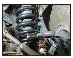
2. Next, slip the spacers between the coils and let them fall into the coil cup. [FIGURE 2]
