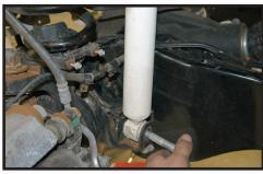
3. Remove track bar bolt at frame. [FIGURE 3]
