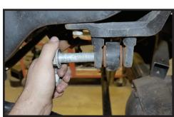
4. Lower front axle until the coils can be removed from vehicle. [FIGURE 4 & 5]
