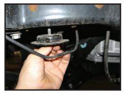
16. Install the driver side coilover: The reservoir hose will point towards the front of the vehicle indicating the driver side. With the reservoir bracket sandwiched between the coil bucket and the coilover mount, use the supplied 3/8" hardware to fasten the coilover to the coil bucket. [Torque to 45 ft-lbs] Twist the hose and loop around to the reservoir mount as shown. Attach the reservoir to the mount using the supplied hose clamps with a 5/16" socket/wrench. [FIGURE 14]
