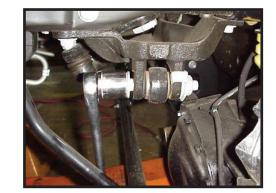
**5.** Support the axle with a floor jack and remove the front shocks. The shocks are limiting droop so make sure that the axle is supported or it will fall when the shocks are removed. (21mm socket/wrench, 18mm socket/wrench)
