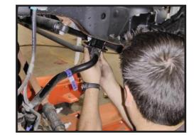
19. Reconnect the sway bar to the stock links using an 18mm. [Torque to factory spec]
