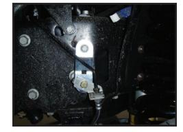
**27.** Remove parking brake bracket from the side of the frame using a 13mm socket/wrench. Mount the drop bracket using the factory hardware. Fasten the wire bracket to the drop bracket using the supplied 3/8" hardware and a 9/16" socket/wrench. **[FIGURE 8 & 9]**
