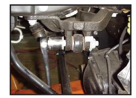
**5.** Support the axle with a floor jack and remove the front shocks. The shocks are limiting droop so make sure that the axle is supported or it will fall when the shocks are removed. (21mm socket/wrench, 18mm socket/wrench)
