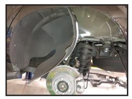
4. Support the lower control arm. Remove the upper coilover nuts using an 18mm. [FIGURE 2]
