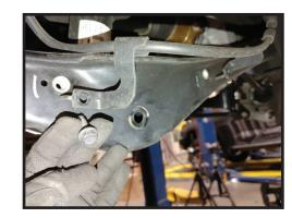
7. Remove the lower control arm bolt and nut using an 18mm. Remove the coilover from the vehicle and set aside. [FIGURE 5 & 6]
