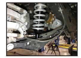
10. Reinstall the brake line bracket and lower control arm pivot bolt. Torque the pivot bolt to 180 ft-lbs.
