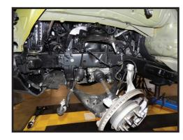
11. Grab the new ICON collover and make sure the lower bar pin is oriented correctly for ease of bolt installation. This may require using an adjustable wrench or vise to rotate the barpin/bearing as shown. [FIGURE 12]
