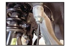
**7**. Now support the knuckle with a strap to the frame to keep it from falling away and pulling apart the CV axle. Then remove the nut from the upper ball joint. The knuckle should rotate out of the way to easier access the coilover.
