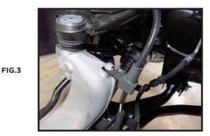
5. Remove the tie rod nut using a 21mm and remove the tie rod of the knuckle using a ball joint separator. [FIGURE 4]
