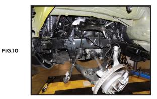
11. Using a 21mm ratchet and 21mm wrench, loosen and remove the upper control arm from the frame mounts (two ratchets are shown but a wrench can be used inside the coil bucket). [FIGURE 11 & 12]
