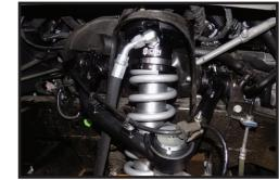
*16.* Secure the harness to the UCA with the supplied M6 hardware and push the clips into the arm. Install dust cover with the supplied
