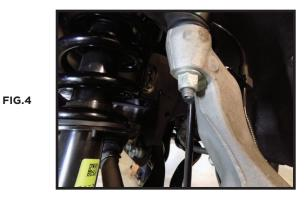
**7.** Now support the knuckle with a strap to the frame to keep it from fall away and pulling apart the CV axle. Then remove the nut from the upper ball joint. The knuckle should rotate out of the way to easier access the coilover.
