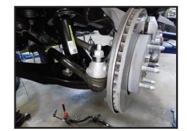
**6.** Next you will need to loosen and remove the upper joint nut using an 18mm. Then use the ball joint separator to break the ball joint taper free from the knuckle. A well-placed hit with a hammer onto the knuckle can also free the taper. Leave the nut attached so the knuckle does not fall away and pull apart the CV joints. [FIGURE 4]
