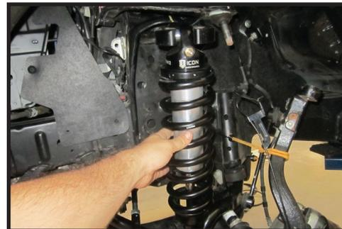
6. Remove the 3 upper nuts securing the stock shock to the bucket. Do not loosen or remove the larger center nut securing the spring seat to the shock shaft!!! This will result in the stock coil assembly to come apart violently, causing damage to components and possible injury!
