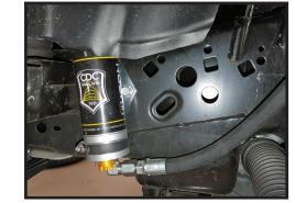
15. Mount the reservoir to the bracket using supplied hose clamps and a flat head screw driver or 5/16" socket/wrench.
