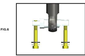
**11.** Connect the upper control arm to the spindle using an 18mm socket/wrench. [Torque OEM balljoint to factory spec] [75 ft-lbs for the ICON DELTA JOINT]
