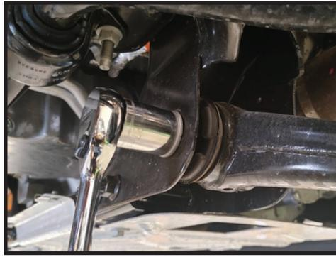
**NOTE:** If you prefer to leave the lower arm in place, use a hammer to push the studs out of the lower bar pin assembly.
