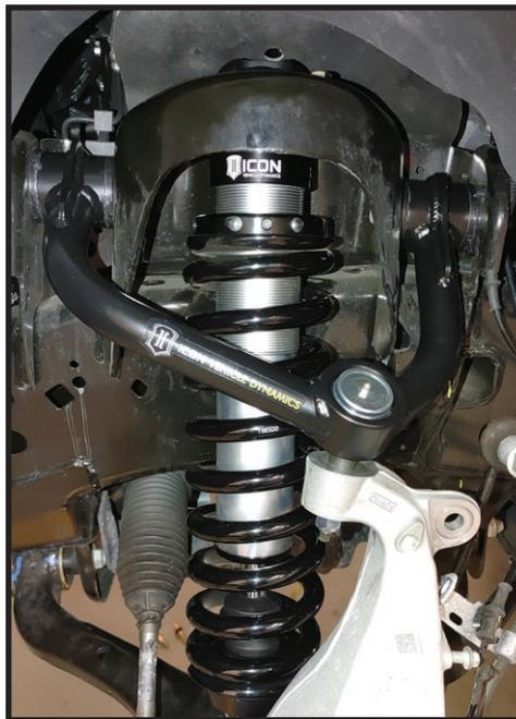
**10.** Use the supplied 7/16" bolts and washers to secure the ICON coil-over to the lower arm using a 5/8" wrench/socket [Torque to 50 ft-lbs]. The bar pin is installed to offset the shock forward to increase axle clearance. Each 7/16" bolt will get 2 washers, the thicker black oxide washer will go against the Lower control arm, while the thinner yellow zinc washer will go against the head of the bolt. [FIGURE 6 & 7]
