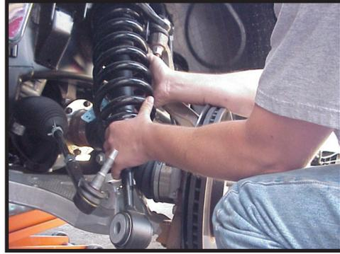
**8.** Before installing the new ICON coilover, the stock coil bucket will need to be trimmed to allow for clearance of the large hose attaching the remote reservoir and compression adjuster. Use the examples to lightly trim the edge to allow the fittings to pass through the bucket. [FIGURE 5 & 6]
