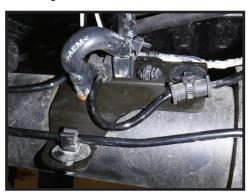
24. Reinstall the wire harness and bracket on the driver side inside frame rail with longer supplied 8mm bolt. There is an oval hole in the inner bracket to accommodate the clip that was removed from the top of the frame. [FIGURE 38 & 39]
