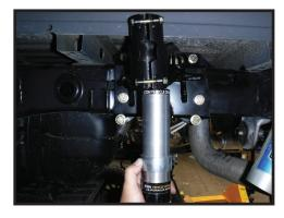
**21.** Install the striker pads on the axle tube. Pop the ABS clip from the tab on the axle tube. The lower portion of the striker plate hooks under the leaf spring pad on the axle. The slot where the ABS tab was will need to be opened up for the bolt that will secure the striker. Standard drill bits will tend to catch in the oval hole, a die grinder is recommended. Tighten until the pad is in full contact with the axle tube but do not overtighten. [FIGURE 30 - 33]
