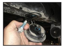
4. Move brake line bracket and wire harness on the driver side. Nothing needs to be disconnected just pushed out of the way. Remove the bolt holding the brake line bracket to the inside of the frame. Using a panel clip tool or large flat screwdriver, pop the plastic retaining clips out of the inside and top of the frame rail. You can now flex the lines and harness away from the inside of the frame. [FIGURE 3 & 4]
