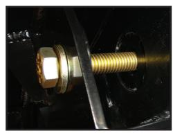
11. Preinstall the two mid plates (PN: 194026, 194027) on the billet crossmember with (2) 1/2"x 2.75" bolts and washers so that the head of the bolts points towards the front of the truck. [FIGURE 17 & 18]
