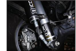
**5.** Install the ICON shock in the lower mount. Firmly press upward on the shock to compress it enough to line it up with the lower mounting hole and start the bolt. Make sure the nuts are properly retained in the sheet metal retainers. When tightening the lower shock bolt push up on the shock as much as possible to prevent contact with the mounting tabs, slight sanding of the mounting tabs may be necessary. Torque upper and lower shock bolts to factory spec using a 15mm. [FIGURE 3]
