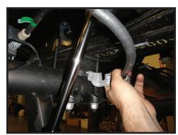
7. Slide the supplied parking brake cable bracket over the metal sleeve on the cable. Connect it to the differential using the factory screw and a 10mm socket/wrench. [Torque to factory spec] [FIGURE 7]
