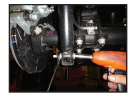
3. The passenger side upper shock mount needs to be sanded slightly in order for the ICON shock to fit. [FIGURE 2 & 3]
