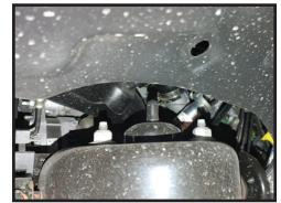
7. If the lower arm was removed, Reinstall it now, only snugging the bolts in place (They will be torqued at the end).
