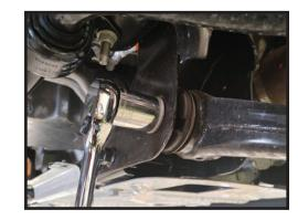
4b. If you prefer to leave the lower arm in place, use a hammer to press the studs out of the lower bar pin assembly.
