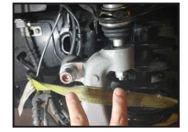
10. Remove the UCA from the frame using a 21mm and 18mm socket/wrench.
