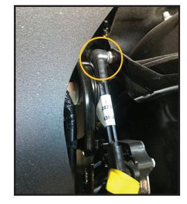
**9.** Remove the sway-bar link and upper control arm from the spindle. Support spindle with a jack or strap to prevent the CV (4x4) or brake lines from over extending (18mm, 21mm, T45 Torx). **[FIGURE 4]**
