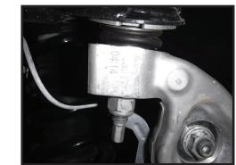
5. Separate the UCA from the spindle and support the spindle so that it does not overextend the CV joints when detached.
