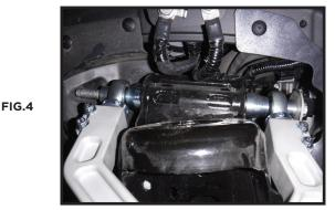
**8**. Pivot the Delta Joint stem so that it is inline with the taper bore in the spindle. The new Delta Joint will be very stiff the first time you move it. Rotate the upper control arm downward and install the stem through the spindle taper. Install two washers per side with the supplied flanged nut on the taper pin. Connect the UCA to the spindle using an 18mm. [Torque to 60 ft-lbs]
