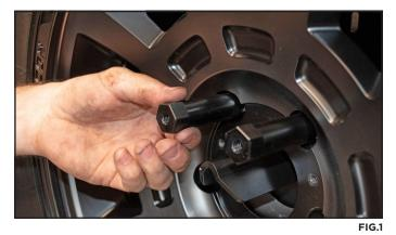
3. Use the two (2) 3/8-16 X 3/4 Gr8 Hex Head Cap Screws, with 3/8 Gr8 SAE Flat Washers, to attach the Mounting Bracket to the two M14 Lug Nut Standoffs. Orient the bracket so that the small flange is on top and pointed toward the wheel, as shown in the photo. Tighten with a 3/8" wrench or socket.
