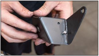
Install your license plate and the Camera Mount/ Cover assembly to the License plate mount simultaneously, with the camera assembly hanging from the bottom two license plate bolts. Use a pair of 7/16" wrenches or sockets and four (4) 1/4-20 X 3/4 SS Button Head Cap Screws with 1/4 Gr8 SAE Flat Washers and 1/4-20 Gr8 Nylon Insert Lock Nuts to fasten the components together.
