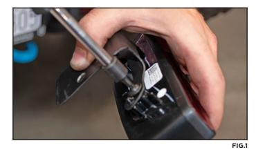
Stack the License Plate Bracket and Brake Light Bracket on top of the Mounting Bracket and fasten them all together with two (2) 5/16-18 X 3/4 Gr8 Hex Head Cap Screws and 5/16 Gr8 SAE Flat Washers. Use a 1/2" wrench to tighten. Note that the License Plate Bracket is slotted to allow adjustment.
