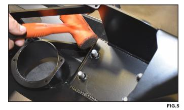
Install a winch fairlead on to the bumper. Begin by checking your fairlead's mounting bolts against the fairlead mounting holes in the ICON bumper. Some fairleads come with larger mounting bolts, in which case the holes in the bumper will need to be drilled to the larger size. If you do this, make sure to use touch-up paint on the exposed metal of the drilled holes.
