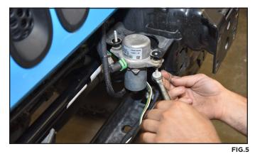
Use a hack saw, die grinder or cutoff wheel to remove the excess threads from the forward-most of the two mounting bolts.
