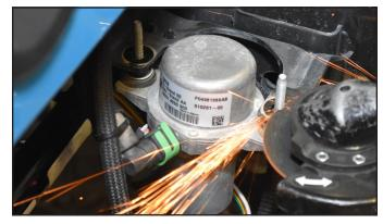
9. If mounting the bumper with a Warn Zeon winch, trim the top-inside corner of the bumper mounting flanges on each frame rail. Begin by marking your cut as indicated by the white line in the image below, leaving about 3/16 to 1/4 of an inch of material around the edge of the bolt hole.
