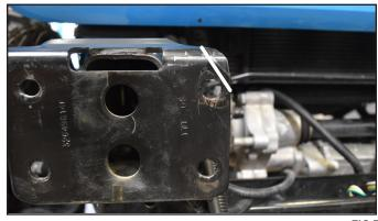
Use a die grinder or cutoff wheel to cut the corner of the bumper mounting flange.
