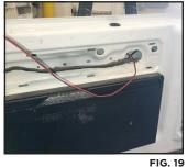
17. Using a pry tool or slightly pulling on the bottom of the trim piece behind the factory jack compartment, remove by lift the trim piece and set aside. Partially remove the trim piece on the passenger side inner wall in the trunk area by slightly pulling on the bottom of the trim.
