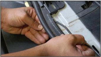
Note: Before continuing this step, you could measure out the distance between the remaining wire lead and the license plate light wire harness and cut the excess wire for a cleaner look, or use cable ties to clean up the wire.
