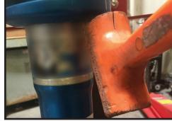
**9.** Position the split preload collar on the shock with the text of the desired lift height right side up (note the lift height indicated assumes the upper shim ring is also used). The bolt heads of the collar should be towards the live valve actuator [Tighten bolts to 12 ft-lbs]. Make sure that the inner locking portion of the collar is securely seated inside the groove on the shock body. [FIGURE 14]
