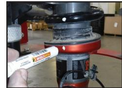
7. It is not necessary to disassemble the shock or coil, however the spring will need to be compressed a couple of inches. A quality spring compressor is necessary; we recommend a three arm style as shown in the photos. [FIGURE 5 & 6]
