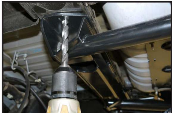
**17.** Use the shock mount as a drill guide to drill into the crossmember with a 1/2" drill bit. Once the holes have been drilled and the inside has been deburred, use the supplied 1/2" (605322) nuts and (605330) washers in bag 1 to tighten the shock mount to the crossmember using 3/4" socket/wrench. (FIGURE 5) [Torque 1/2" hardware to 80 ft-lbs, and factory hardware to factory spec]
