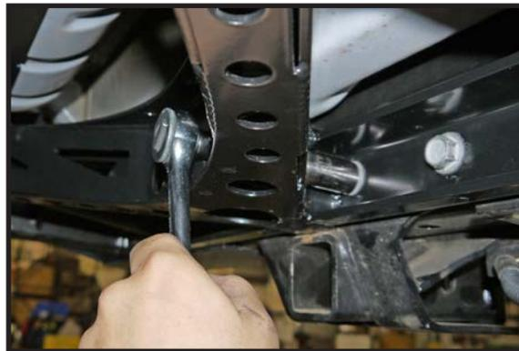
**16.** Use a c-clamp to pinch the other end of the shock mount to the crossmember over the rear axle. (FIGURE 4) Use an 18mm socket/wrench to secure the shock mount to the rear crossmember if using the supplied 1/2" hardware in bag 1. Be sure to keep the mount flat against the surface and the edges parallel to the frame.
