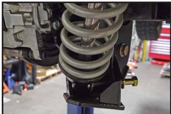
**24.** Tighten all hardware on the axle mount. (FIGURE 10) [3/8" > 45 ft-lbs] [1/2" > 90 ft-lbs] [9/16" > 110 ft-lbs]
