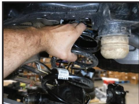
**9.** Install the multi-rate coil spring. Ensure the upper coil isolator is located properly on the coil and the locator nipple is in the locating hole in the frame. [FIGURE 8 & 9]
