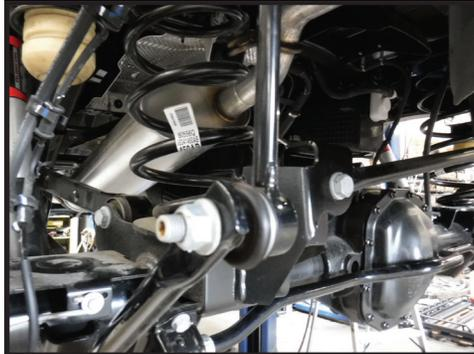
6. Disconnect the brake line bracket from the side of the frame using a 10mm. [FIGURE 4 & 5]
