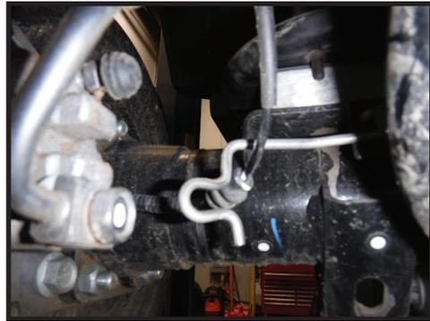
**11.** Connect the ABS wire to the retainer on the differential.
