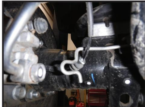
7. Disconnect the ABS line from the wire retainer on the differential.
