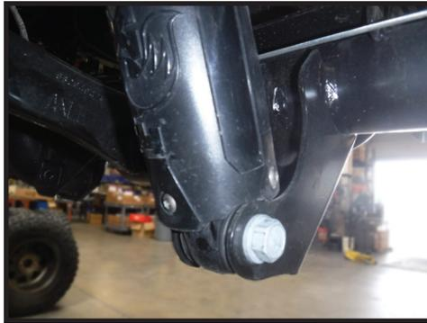
5. Disconnect the rear sway bar from the frame using an 18mm. [FIGURE 3]
