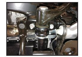
5. Support the lower control arm and remove the bolts from the frame. Remove the 15mm nuts from the top of the coilover. [FIGURE 4]
