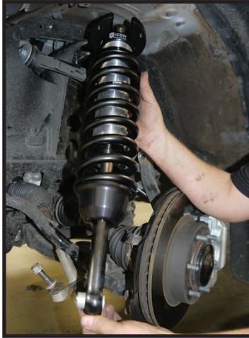
**8.** Connect the shock to the lower control arm: The lower shock mount has (1) long and (1) short spacer [Torque to factory spec]. Make sure the long spacer is toward the front of the vehicle as this will position the shock further toward the rear of the control arm to ensure adequate sway bar clearance. Install the factory lower shock bolt.
