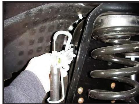
**3.** Disconnect the upper brake line brackets from the frame using a 13mm and lower brake line brackets from the differential using a 10mm. [FIGURE 2]
