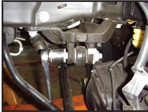
5. Support the differential with a floor jack and remove the front shocks. The shocks are limiting droop so **MAKE SURE THE AXLE IS SUPPORTED OR THE AXLE WILL FALL** when the shocks are removed. Use an 18mm on the bottom and a 16mm on the stem of the shock.
