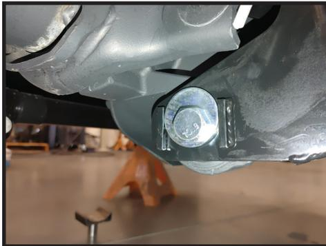
**8.** Install the supplied M18 x 130mm bolt with 1 washer into the upper hole and mount. No washer on the inside as there is not enough room between the nut and the differential housing. [FIGURE 6]
